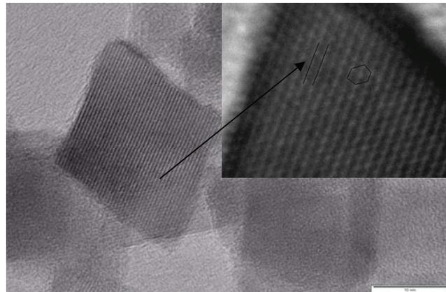
Figure 2: Typical bright field TEM image showing welding fume particles with rhombohedral morphology and lattice fringes. The inset image is at higher magnification, showing the lattice fringes more clearly.
