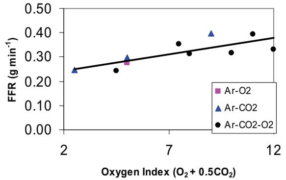
Figure 4: FFR plotted against oxygen index for the Ar-O<sub>2</sub>, Ar-CO<sub>2</sub> and Ar-CO<sub>2</sub>-O<sub>2</sub> series.
