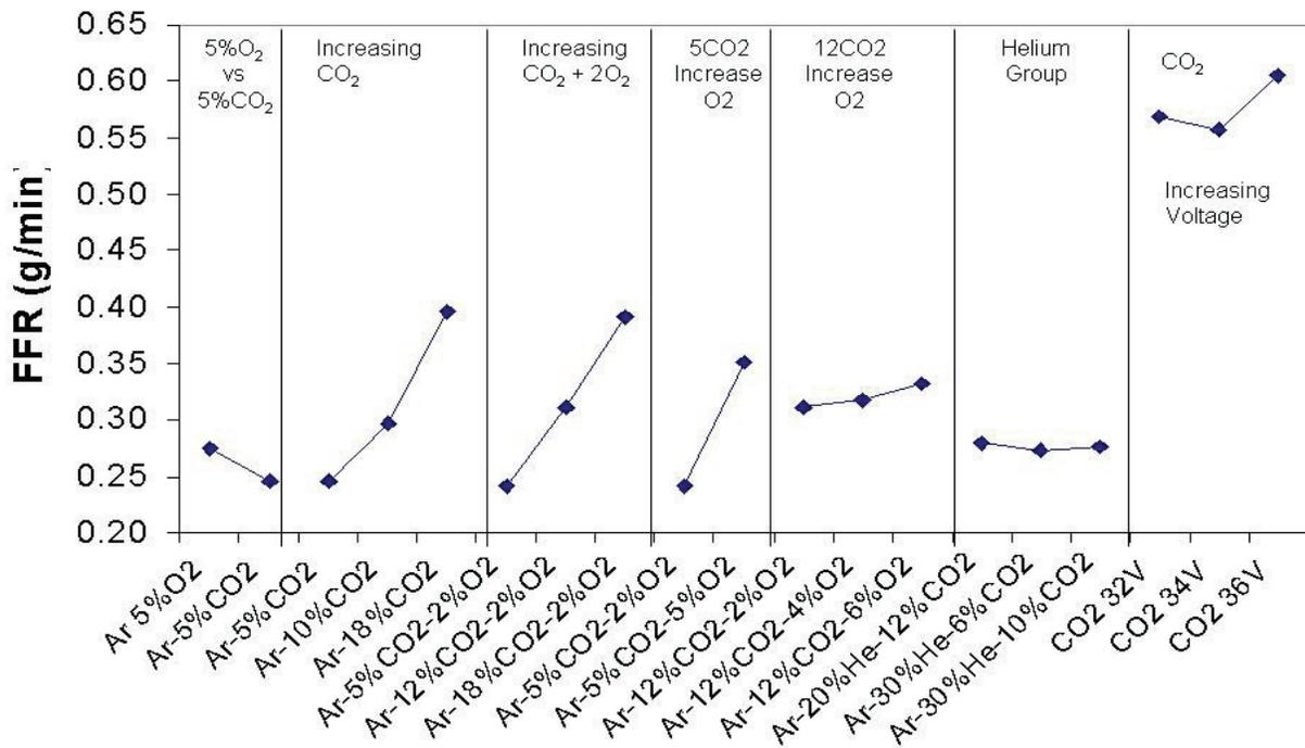
Figure 3: FFR as a function of shielding gas composition under the same welding conditions. Each region on the graph groups the shielding gas mixtures according to different variables in the composition.
