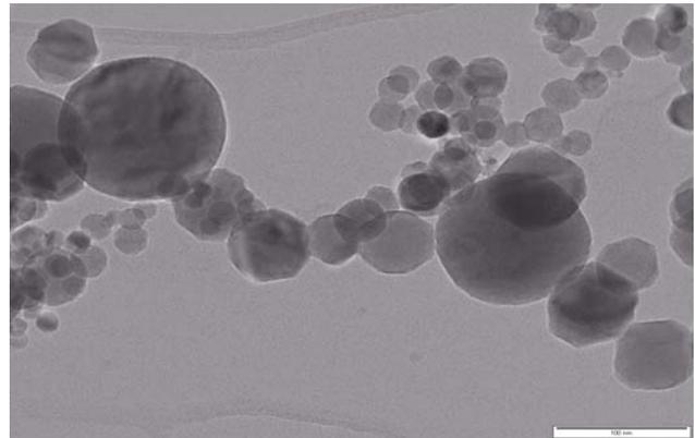
Figure 1: Typical bright field TEM image showing welding fumes with a mixture of particle sizes, with either spherical or faceted morphology and often in chain-like structures.
