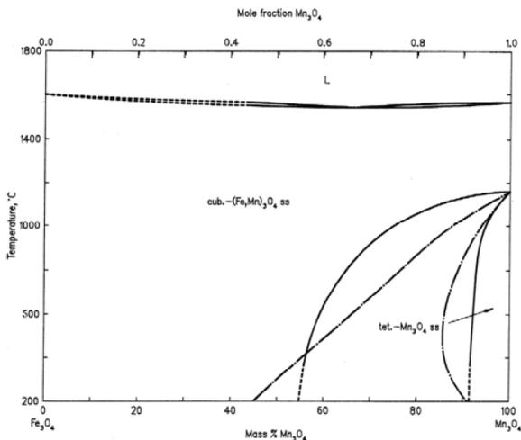
Figure 6:  $Fe_3O_4$ - $Mn_3O_4$  system, showing an extensive region of cubic  $(Fe,Mn)_3O_4$  solid solution, reproduced from the Slag Atlas.<sup>27</sup>
