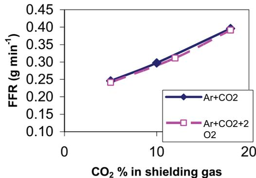
Figure 5: FFR plotted as a function of CO<sub>2</sub> in shielding gas for Ar-CO<sub>2</sub> and Ar-CO<sub>2</sub>-2%O<sub>2</sub>.
