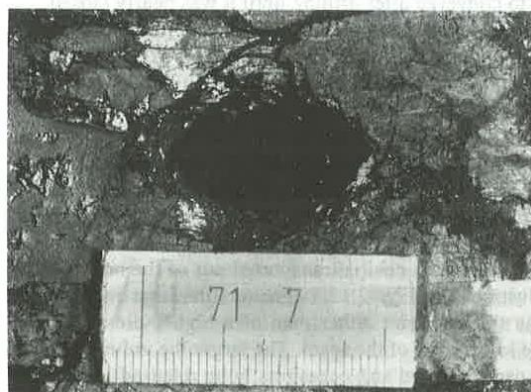
Figure 5: Borehole coalburst, an example of the loss of confinement mechanism (Brauner 1994)
