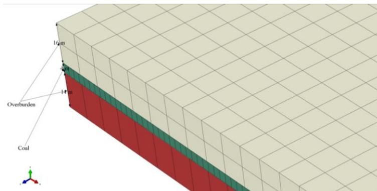
**Figure 1: Illustration of a typical single pillar model**
