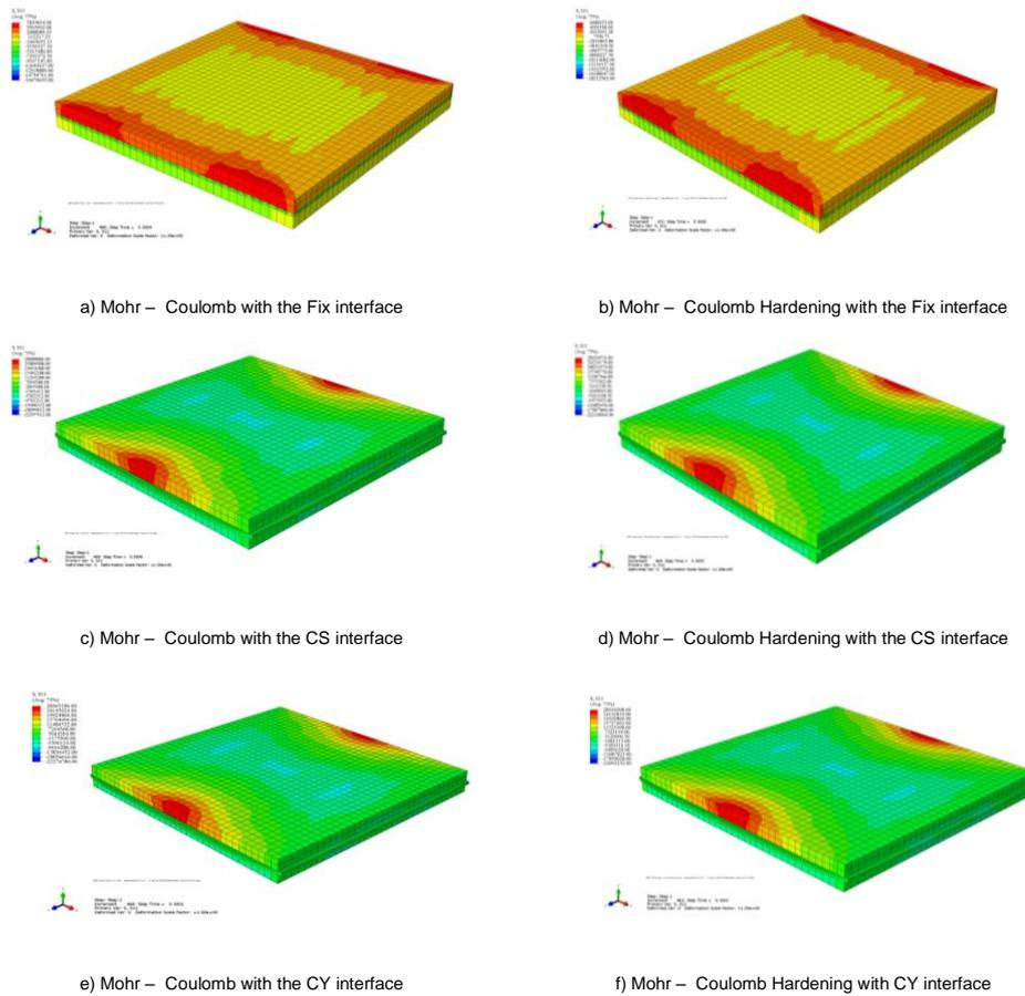
**Figure 4: Stress distributions due to the different material and joint properties**
