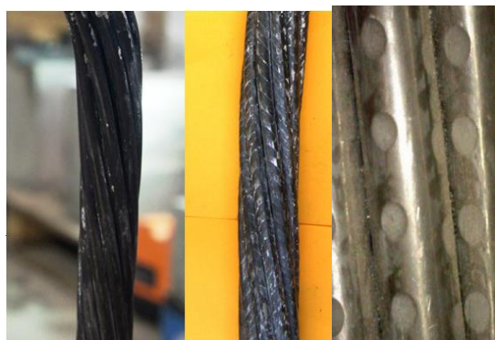
Figure 1: Cable bolts profile: plain, spiral and indented
