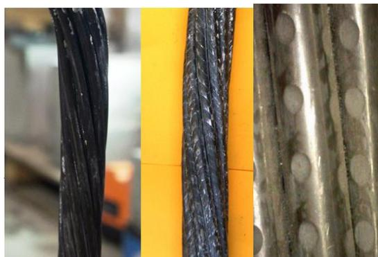
Figure 1: Cable bolts profile: plain, spiral and indented
