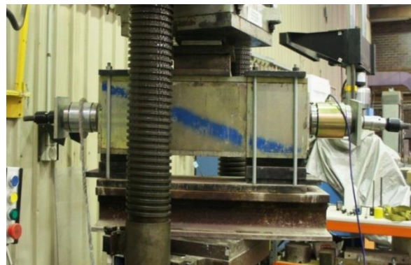
Figure 7: Arrangement of the cabled concrete blocks in 500t machine (Aziz et al. , 2015)
