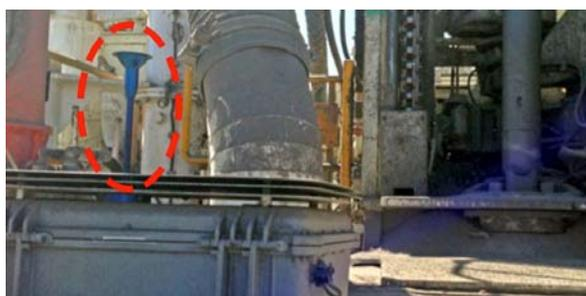
**Figure 3: Dust monitor in use during drilling operations**
