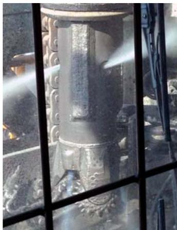
**Figure 2: Water spray from weep holes in side of the sub above the drill bit**
