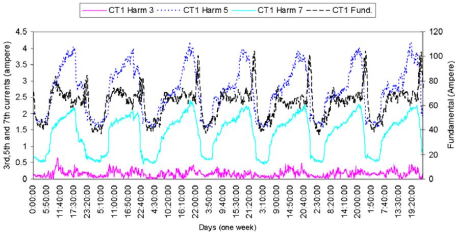
Fig. 3. Residential feeder (Site 2) weekly harmonic Current data from the monitoring equipment.
