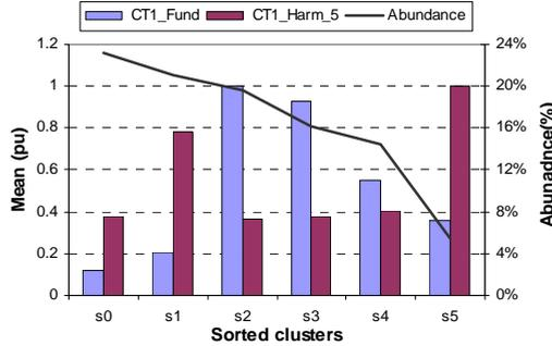
Fig. 5. Fundamentals and 5<sup>th</sup> harmonic current clusters in a single phase.
