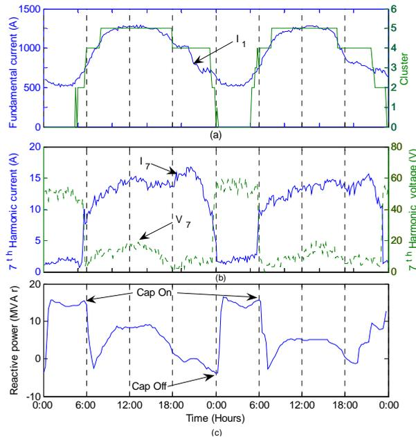
Fig. 16. Clusters at substation site in two working days (a) Clusters superimposed on the fundamental current waveform, (b) 7<sup>th</sup> harmonic current and voltage data. (c) MVAR load at the 33kV.
