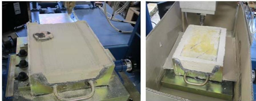
Figure 2: Method of securing the blocks of rock samples for cutting tests
