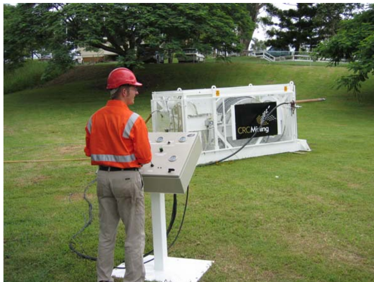
Figure 7: CRCMining's prototype HSXP rig with 350m hose capacity (2005)
