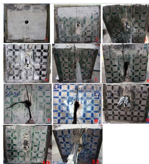
Figure 9: Concrete block surfaces after shearing
