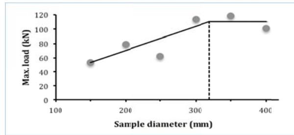
Figure 15: Variation in maximum load with test sample diameter at a bolt torque of 80 Nm
