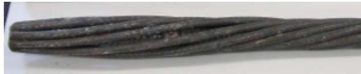
**Figure 3: Sumo strand cable bolt**
