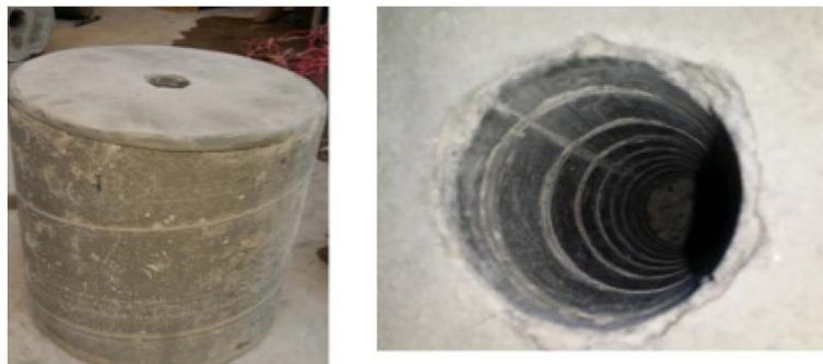
**Figure 6: Test sample (left) with rifling borehole (right)**
