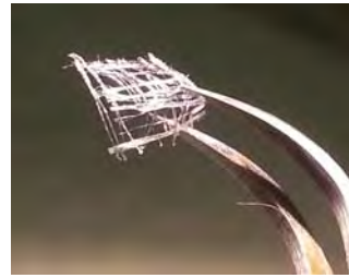
Figure 6: Multi-layered, wet-spun mesh of 1% wt/v alginate containing 20M cells/mL.
