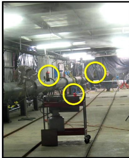
Figure 2 - Positions of CO sensors during the experimental setup showing low-level readings
