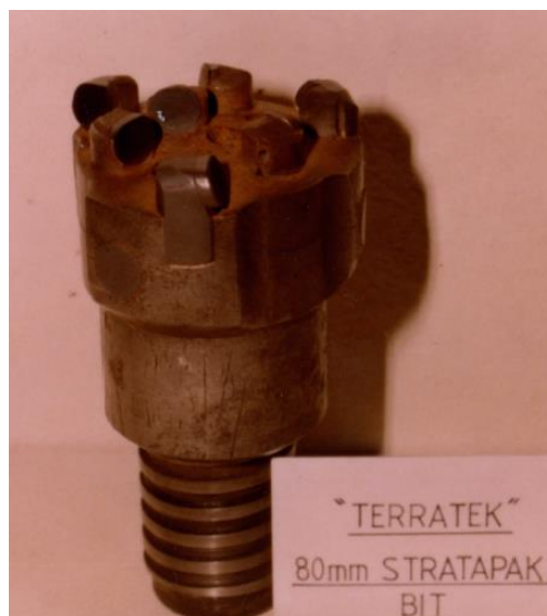
Figure 1 - “Terratek” 80 mm Stratapax PCD bit (Allen, 1982)
