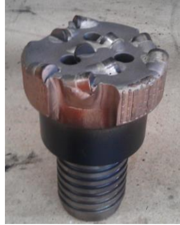
Figure 19 - DPI flat-faced PCD bit with 50% recessed 13 mm cutters
