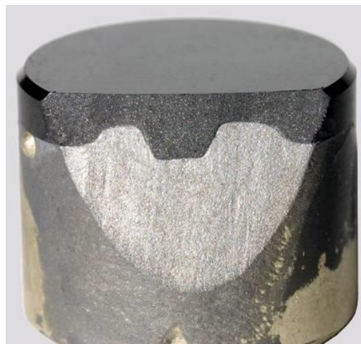
Figure 10 - Progressive wear of a PCD cutter
