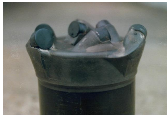
Figure 17 - Modified Longyear 89 mm DHM PCD bit
