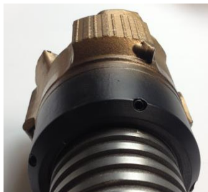
Figure 22 - DPI bit with PCD back-cutters and flushing ports
