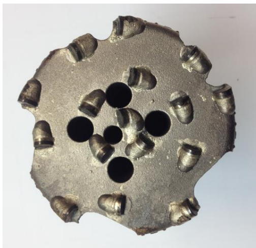
Figure 9 - Flat faced bit with spiral layout of 8 mm PCD cutters
