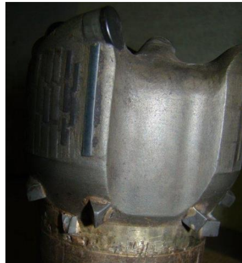
Figure 21 - Asahi PCD bit with tungsten carbide back-cutters
