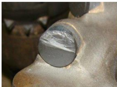
Figure 5 - Fractured PCD table with eroded tungsten carbide substrate
