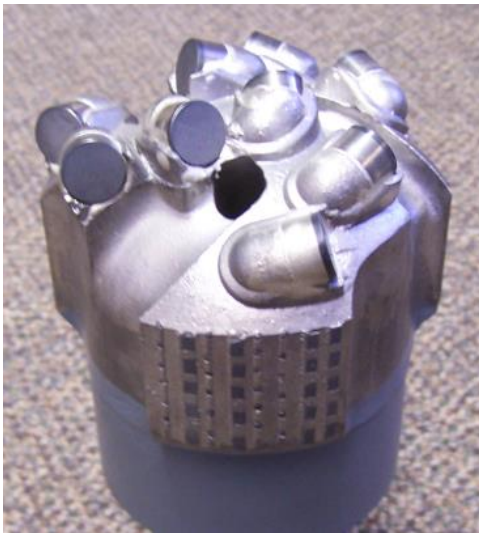
Figure 20 - DPI convex-faced PCD bit with fully exposed 13 mm cutters
