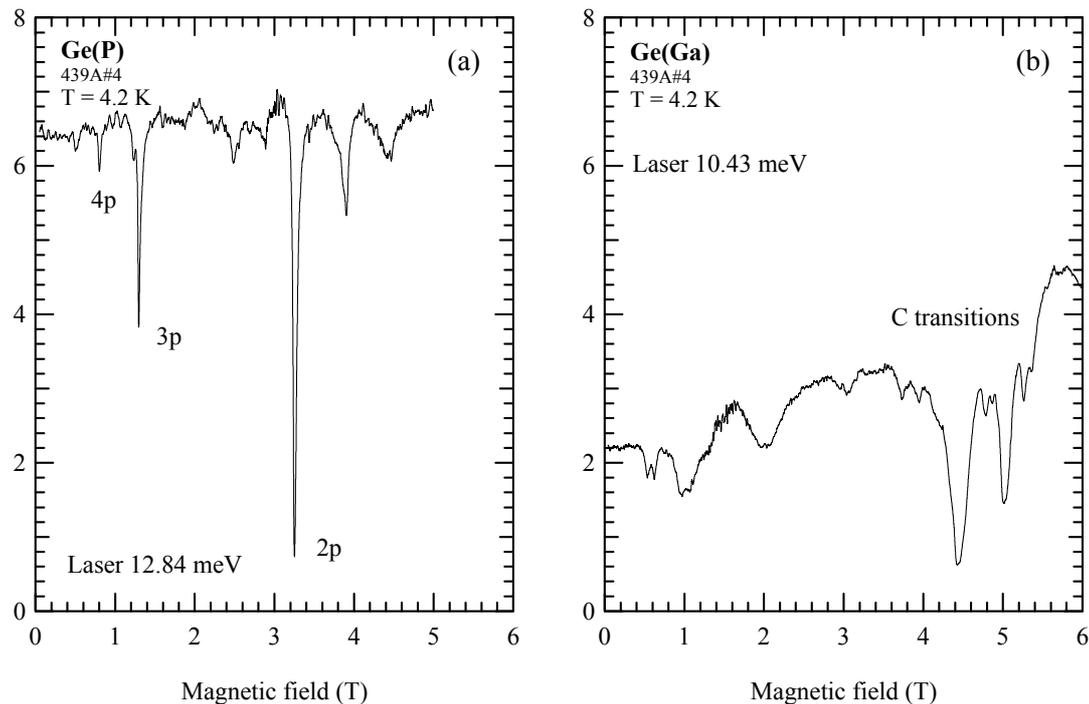
Fig. 2. Transitions of impurities in Ge for  $\mathbf{E} \perp \mathbf{B} || [001]$  determined by FIRL absorption. (a) Laser energy 12.84 meV, detecting Ge(P) transitions. (b) Laser energy 10.43 meV, detecting Ge(Ga) transitions. Vertical axis is absorption (au).
