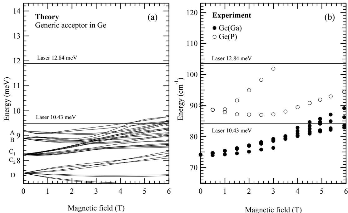
Fig. 1. Transitions of impurities in Ge for  $\mathbf{E} \perp \mathbf{B} \parallel [001]$  from (a) theory [5] (generic acceptor) and (b) experiment [10] (Ga acceptor and P donor). The horizontal lines are laser energies used to obtain the spectra in Fig. 2; in (a) these are adjusted by the central-cell correction.
