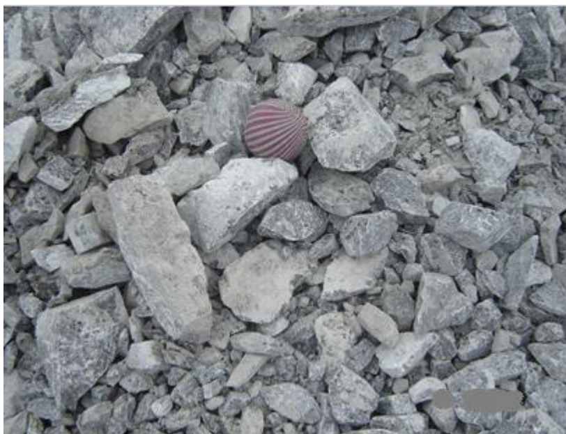
Figure 3 - An example of acquired digital image for calculating size distribution
