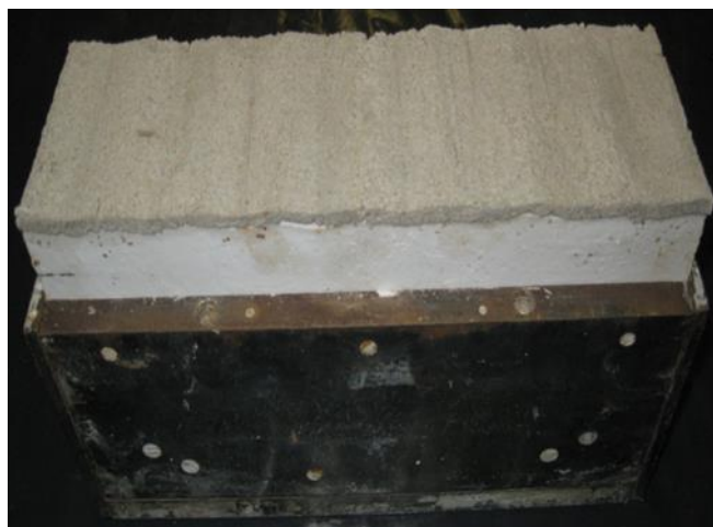
Figure 2 - A close view of artificial infilled joint prepared for testing
