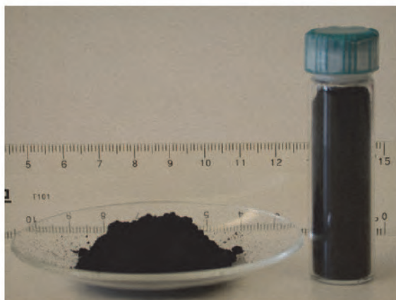
Fig. 3. Example of the bulk quantity of graphene product. The image consists of approximately 2 g of sample (Choucair, M. et al., 2009).
