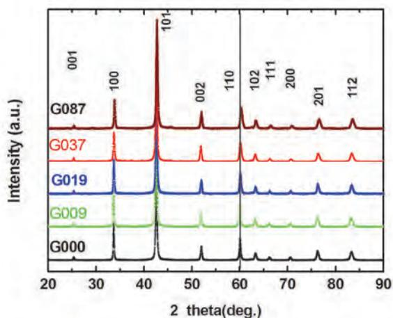
Fig. 4. XRD patterns for graphene doped  $\text{MgB}_2$  samples: G000, G009, G019, G037, and G087, showing that all diffraction peaks can be indexed to  $\text{MgB}_2$  with undetectable impurity phases.
