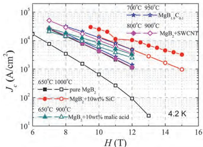
Fig. 2. The critical current density ( $J_c$ ) at 4.2 K versus magnetic field for wires of pure  $MgB_2$  and  $MgB_2$  doped with C, SiC, SWCNTs, and malic acid that were sintered at different temperatures (Dou et al., 2002; Yeoh et al., 2006; Dou et al., 2007; Kim et al., 2008)
