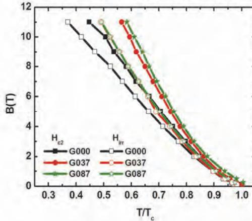
Fig. 10. Upper critical field,  $H_{c2}$ , and irreversibility field,  $H_{irr}$ , versus normalised transition temperature,  $T_c$ , for all graphenedoped and undoped  $MgB_2$  samples (Xu, X. et al., 2010).
