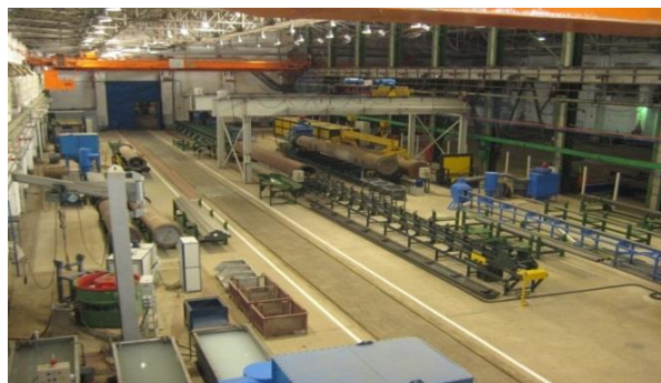
Figure 2 - A modern thermal diffusion galvanising plant, capable of handling products up to 12 metres in length
