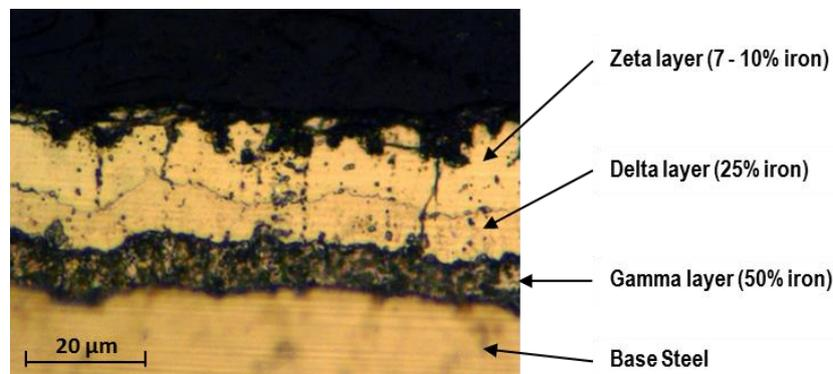
**Figure 4 - A typical thermal diffusion galvanized microstructure. Note the more fully alloyed microstructure and absence of the Eta free zinc layer (ArmorGalv, 2009)**
