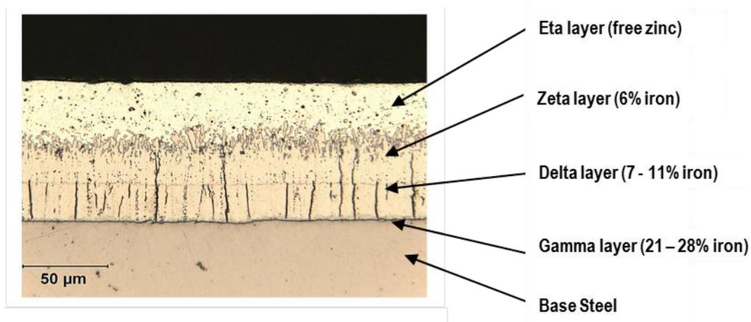
**Figure 3 - A typical hot dip galvanized coating microstructure on structural steel (Industrial Galvanizers, 2006)**
