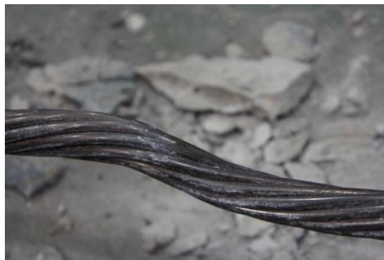
Figure 8 - Post test plain strand cable. No strand failure
