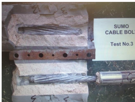
Figure 7 - Test sample after pull test and splitting of the core (Golders UK)
