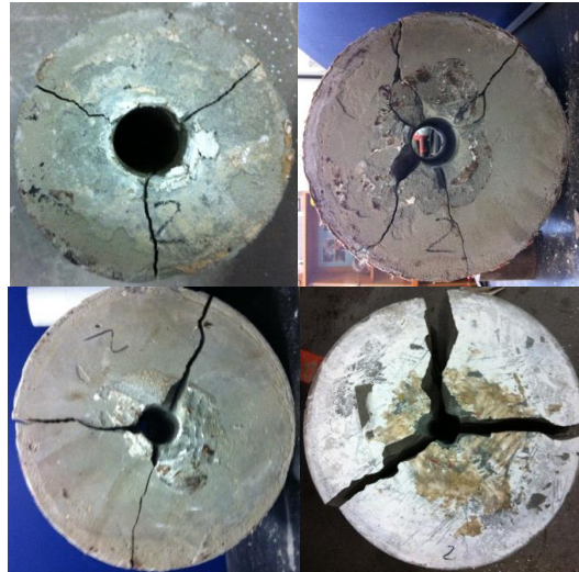
Figure 7 - Evidence of radial tension cracking across all rock cylinder diameters
