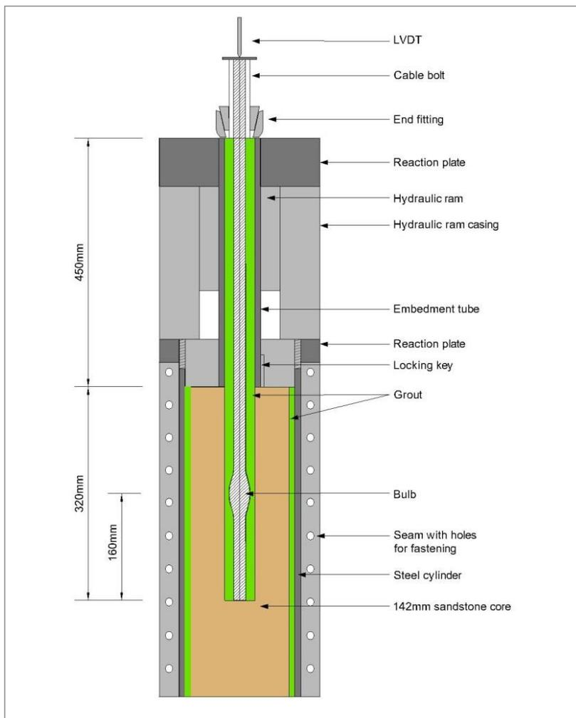
Figure 2 - Modified version of the laboratory short encapsulation pull test incorporating a steel cylinder (Thomas, 2012)
