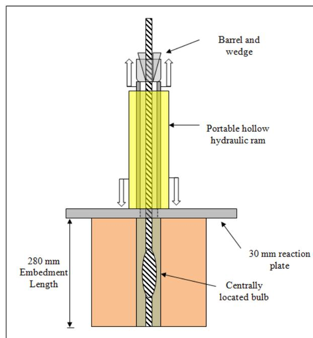
**Figure 5 - Schematic of pull testing arrangement using hydraulic cylinder**
