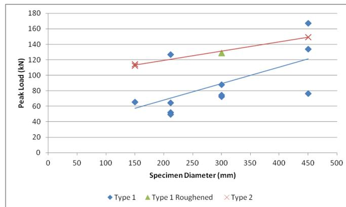
**Figure 6 - Variation in peak load with cylinder diameter**
