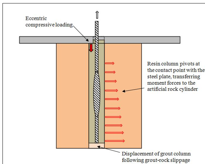
Figure 9 - Schematic of eccentric loading failure mechanism
