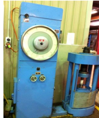
Figure 2 - Uniaxial compressive test set-up
