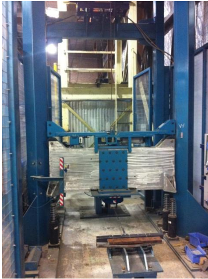
Figure 4 - instrumented drop hammer facility
