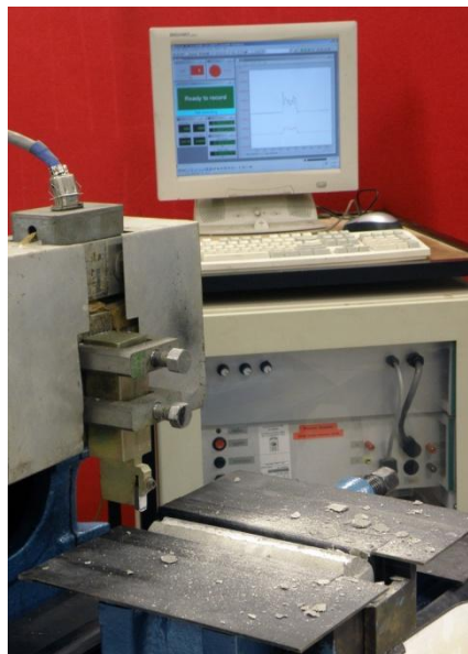
Figure 2 - Instrumentation used in the core cuttability test procedure at UNSW
