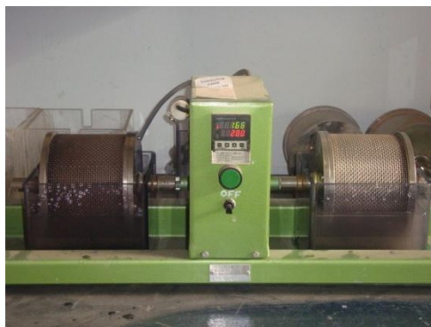
Figure 1 - Slake durability index test apparatus
