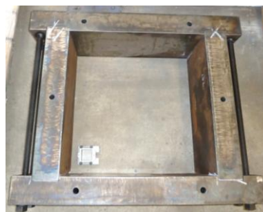
Figure 10 - Scale comparison: Internal shear box of large direct shear machine, with a standard size shear box inset
