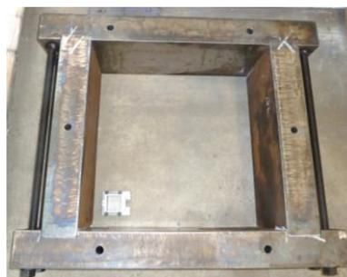
**Figure 10 - Scale comparison: Internal shear box of large direct shear machine, with a standard size shear box inset**
