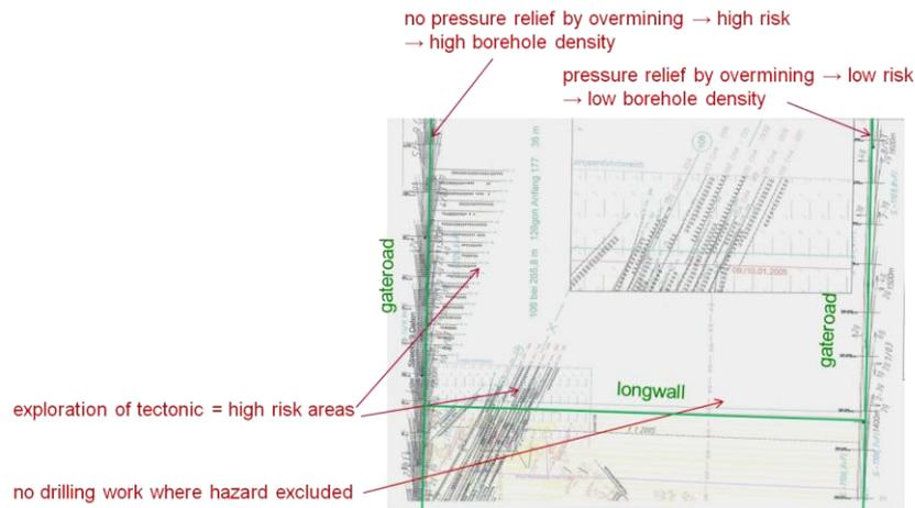
**Figure 2 - Selective exploration and pressure relief drilling**
