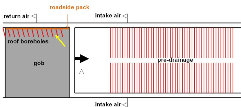
**Figure 7 - Roof borehole layout at Y ventilation system**
