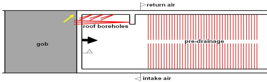
Figure 4 - Typical gas drainage layout at Chinese mine
