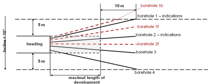
**Figure 3 - Pressure relief drilling (Kunz and Imgrund, 2010)**
