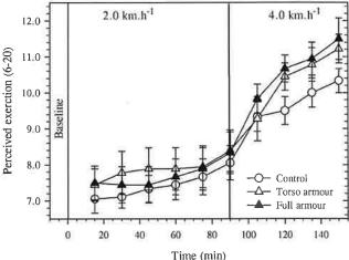
**FIGURE 4.** Perceived exertion (effort sense) during two intensities of steady-state exercise in hot-humid conditions (36°C, 60% relative humidity, and radiant heat ~750 Wm<sup>-2</sup>) while wearing different uniform and body armor configurations.
