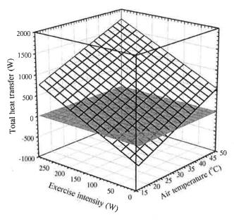
**FIGURE 1.** A predicted transfer surface for a 78-kg individual wearing a single layer of camouflaged, combat fatigues (insulation 0.29 m² K W-1), working at external work loads that may be encountered in the field (rest to 300 W), and exposed to a 35°C ambient temperature range (60% relative humidity). Regions above the zero heat transfer plane represent situations of positive heat storage for combinations of external work rate and air temperature.
