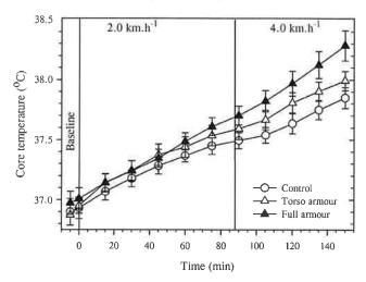
**FIGURE 2.** Core (auditory canal) temperatures during steady-state walking at two speeds in a hot-humid environment (36°C, 60% relative humidity, and radiant heat ~750 W m<sup>-2</sup>) wearing three different uniform and combat armor configurations.
