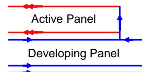
**Figure 6b - Additional intake air from next panel**
