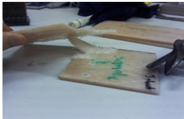
Figure 10 - Delamination along the glass fibre layers
