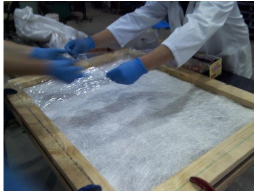
Figure 2 - Preparation of the polymer based glass reinforced TSL
