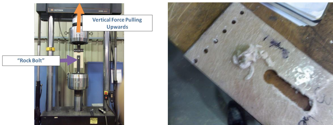
Figure 3 - The polymer sheet with steel rock bolt clamped into the 500 kN Instron servo-hydraulic universal testing machine and teared appart
