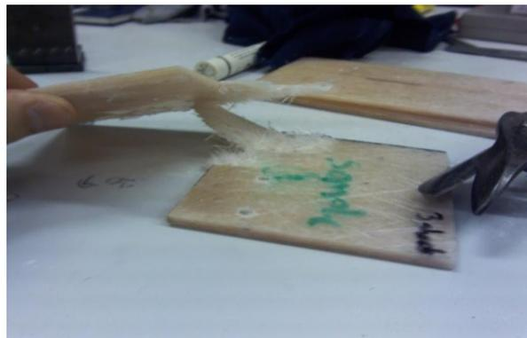
**Figure 10 - Delamination along the glass fibre layers**
