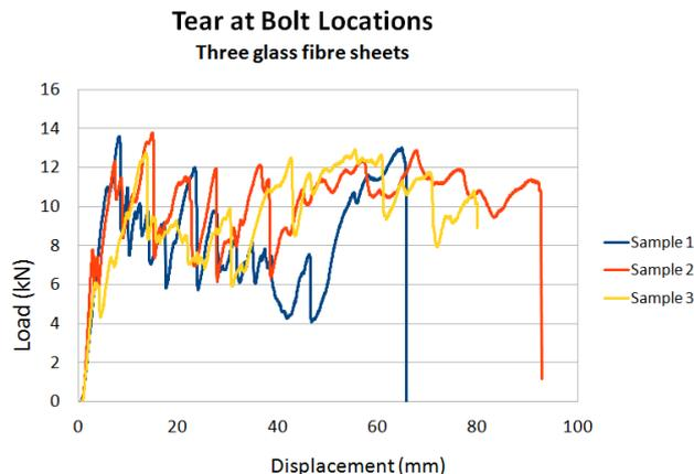
Figure 5 - The measured bolt tearing capacity of polymer samples reinforced with three glass fibre sheet
