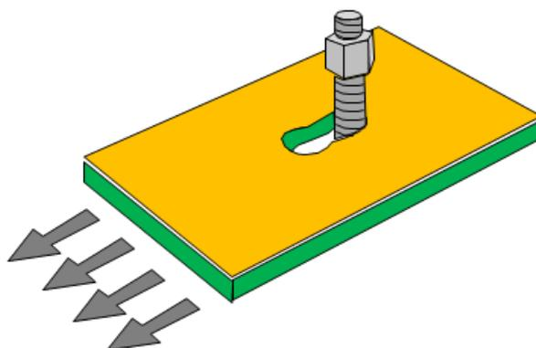
Figure 1 - Schematic diagram of the TSL tearing test
