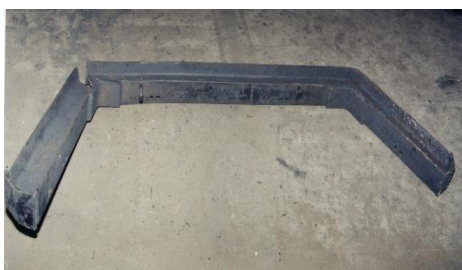
Figure 2 - Support crater cracking
