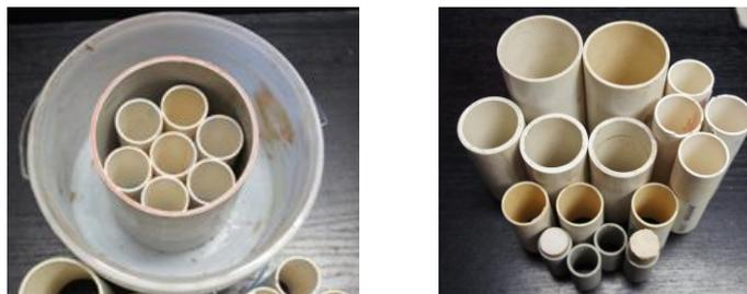
**Figure 1 - Various plastic pipe section moulds and typical moulds arrangement in mixing container. Note two samples in mould**
