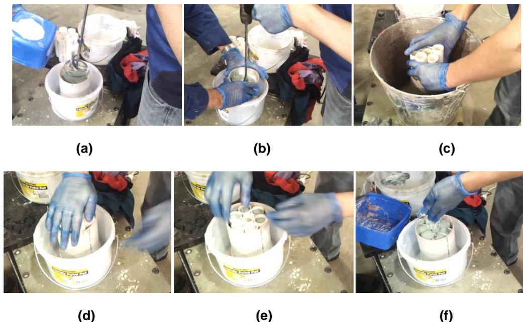
**Figure 2 - Stages of resin mixing mechanically and sample casting in seven moulds simultaneously**
