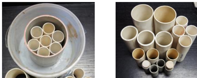
Figure 1 - Various plastic pipe section moulds and typical moulds arrangement in mixing container. Note two samples in mould
