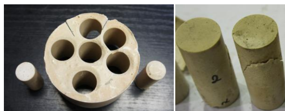
Figure 3 - Mould of slow setting resin and two 20 mm diameter samples
