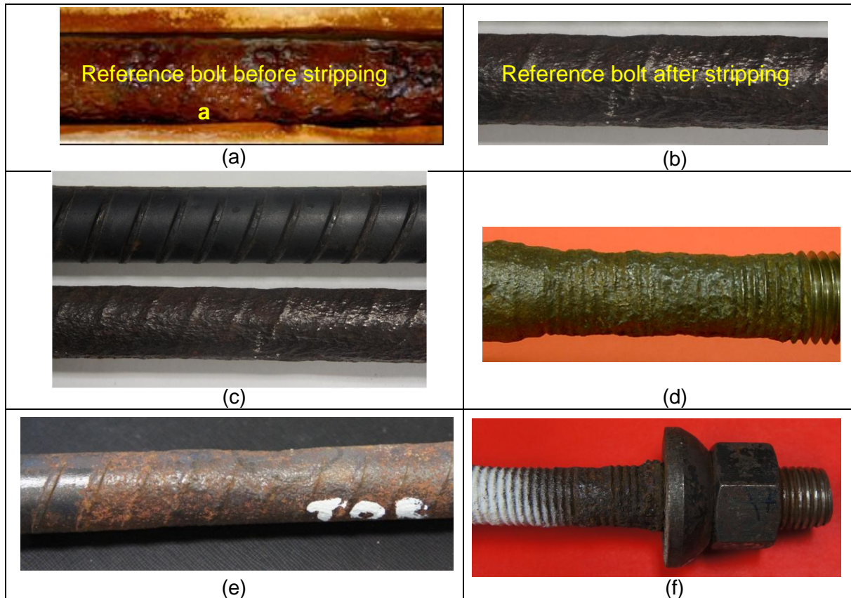
Figure 5 - Photos of parts of various corroded bolt sections compared with un- corroded section. Section (e) shows the evidence of crevice corrosion due to aeration at bolt end
