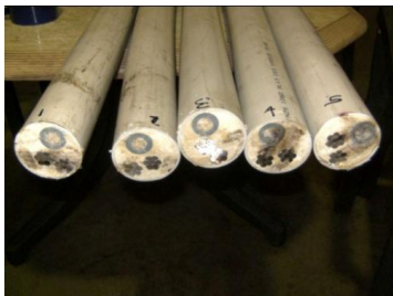
Figure 3 - Cross-section of 6 m twin strand cables
