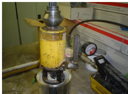
Figure 9 - The laboratory test set-up for pul testing of cables
