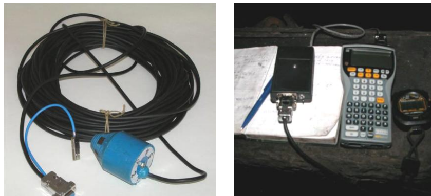
Figure 3 - A gauges probe for long-term measurement of stress tensor changes (left side), registration unit PSION (right side)
