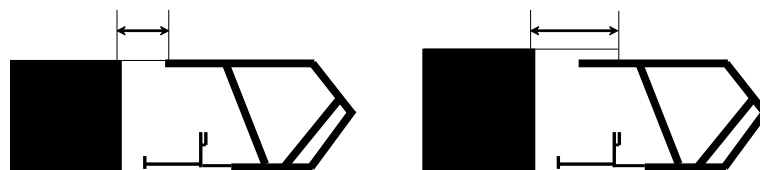
Figure 2 - Illustration of the impact of "steps" in the roof on effective tip to face distance
