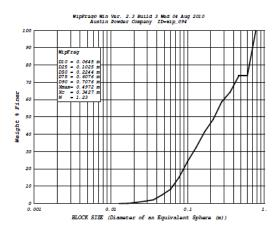
Figure 9 - Fragment size distribution of muckpiles of test blasts with Emulsion explosive
