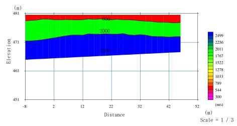
Figure 7 - V<sub>p</sub> profile of major cluster of layers of sand stone strata at bench-III
