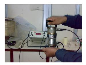
Figure 2 - P-wave velocity determination of sandstone samples from Laboratory testing
