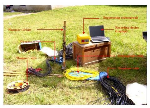
Figure 1 - Various components of the refraction seismic survey system
