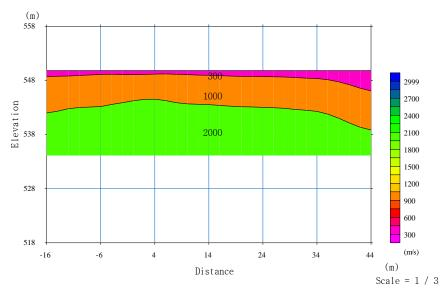
Figure 5 - Vp profile of major cluster of layers of sand stone strata at bench-l
