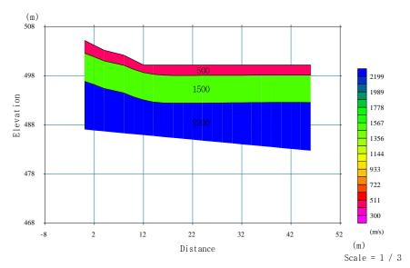
Figure 6 - Vp profile of major cluster of layers of sand stone strata at bench-II
