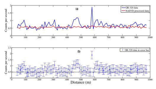
Figure 6 - (a) Gamma ray survey result of the U window along the whole transect with the comparison of the NASVD processed data; (b) Gamma ray result of the U window with error bars, and the dot black line shows the benchmark
