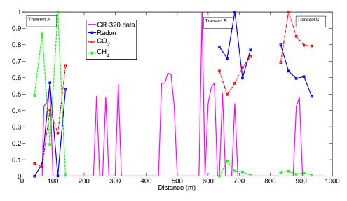
Figure 3 - Radon, CO<sub>2</sub>, CH<sub>4</sub> and GR-320 measurement values are normalized. Gamma ray data from the U window represents <sup>214</sup>Bi signals. The squares show the measuring points.
