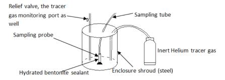
Figure 2 - Schematic of the tracer gas method
