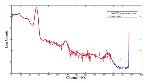
Figure 5 - The comparison of NASVD processed spectra with original spectra
