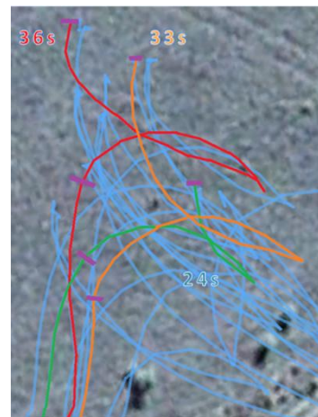
Figure 12 - Spot attempts at the loader of truck 312 on night shift
