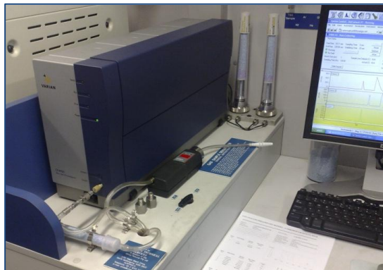
Figure 2 - A typical ultra fast gas chromatograph installation
