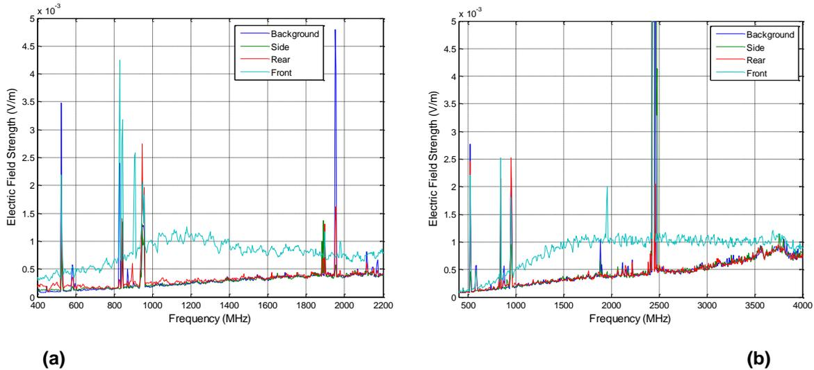
**Figure 3 - Measured electric field strengths for the (a) 900 MHz and (b) 1500 MHz GPR antennas. The maximum electric field strengths from these GPR systems are well below the ARPANSA limits of 47 260 x 10<sup>-3</sup> V/m (900 MHz antenna) and 56 490 x 10<sup>-3</sup> V/m (1500 MHz antenna).**
