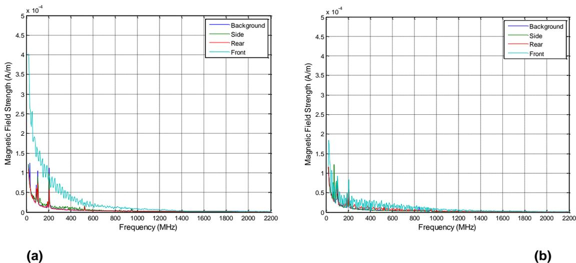
**Figure 4 - Measured magnetic field strengths for the (a) 900 MHz and (b) 1500 MHz GPR antennas. The maximum magnetic field strengths measured from these GPR systems are well below the ARPANSA limit of 729 x 10<sup>-4</sup> A/m.**
