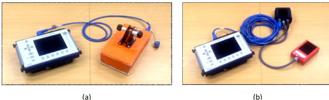
**Figure 3 - Commercial GPR equipment under test. The equipment includes the (a) GSSI 900 MHz antenna (orange unit) and (b) GSSI 1500 MHz antenna (red unit). The display unit on the left side of each image is the GSSI SIR-3000 control unit.**
