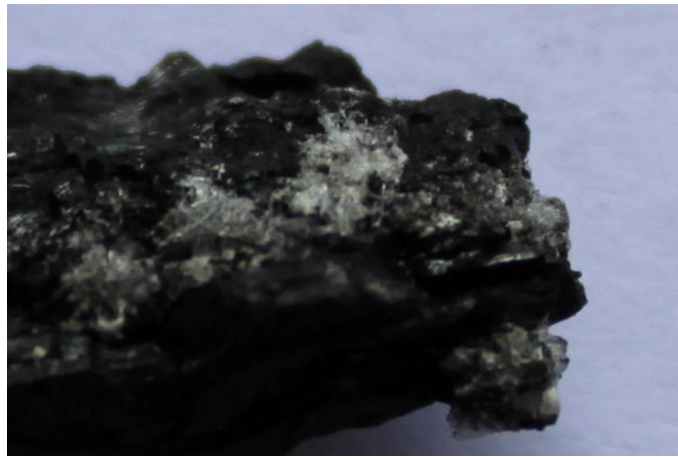
Figure 5 - Bowen Basin high volatile bituminous coal sample showing crystal clusters of hydrated iron sulphates on exposed surfaces
