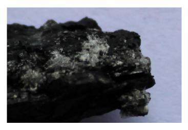
Figure 5 - Bowen Basin high volatile bituminous coal sample showing crystal clusters of hydrated iron sulphates on exposed surfaces
