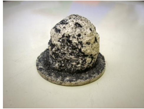
Figure 3b - Shape of cavity by pouring plastic into the cavity after the outburst experiment
