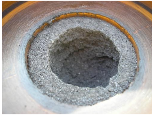
Figure 3a - Formation of cavity in laboratory model outburst experiment
