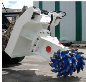
**Figure 9 - QDS attached cutter head**
