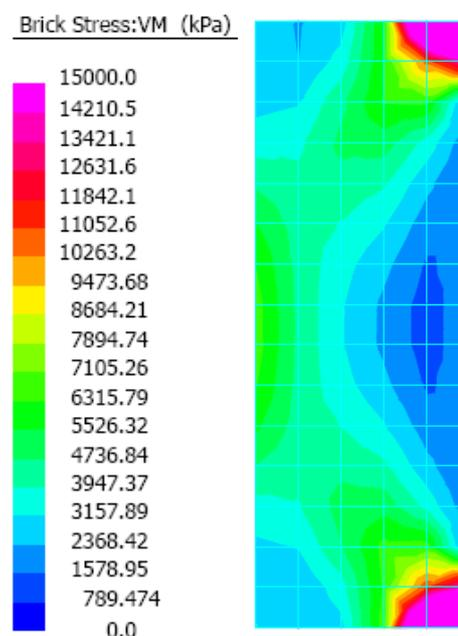
Figure 11 - Stresses in vertical wall section
