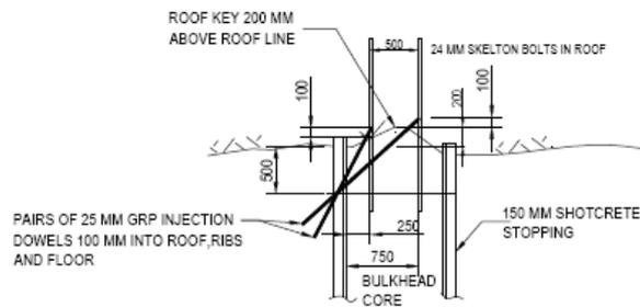
**Figure 8 - Bulkhead roof cross-section showing V shaped roof key and the position of GRP injection dowels in relation to the roof contact**
