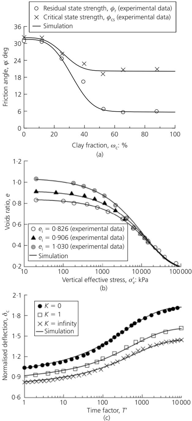
**Figure 1.** (a) Variation of the strength of soil with clay fraction (data after Lupini *et al.* (1981)). (b) One-dimensional compression behaviour of Quiou sand (data after Pestana and Whittle (1995)). (c) Time–deflection of circular raft with flexibility  $K$  (theoretical data after Booker and Small (1984))
