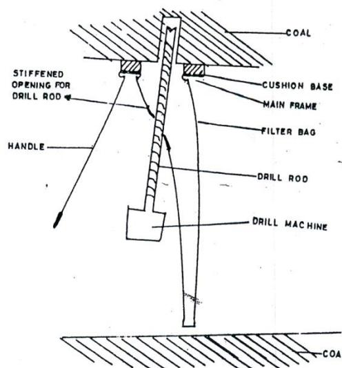
Figure 3 - Dust collector for drilling in mine roof (not to Scale)
