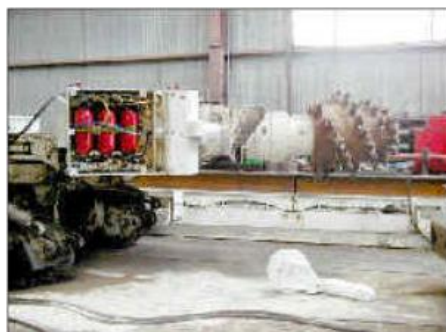
Figure 7 - The Explo-Stop® on-board active suppression system on a Dosco 1300H
