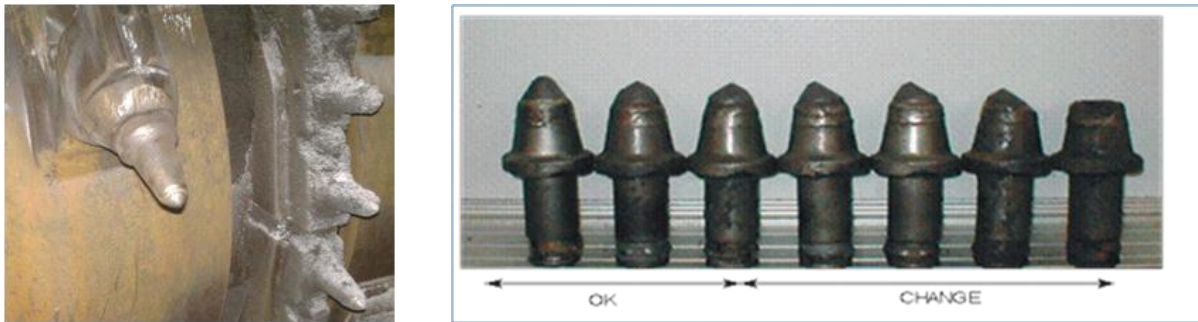
Figure 5 - Cutter head with picks (left) and Pick condition reference guide (right)
