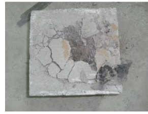
Figure 13 - Fragmentation pattern (25 MPa)
