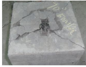
Figure 12 - Fragmentation pattern (50 MPa)
