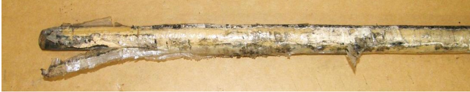
(b) Standard bolt, site 2:1 water based resin - extensive gloving with plastic film intact along 600 mm of bolt
