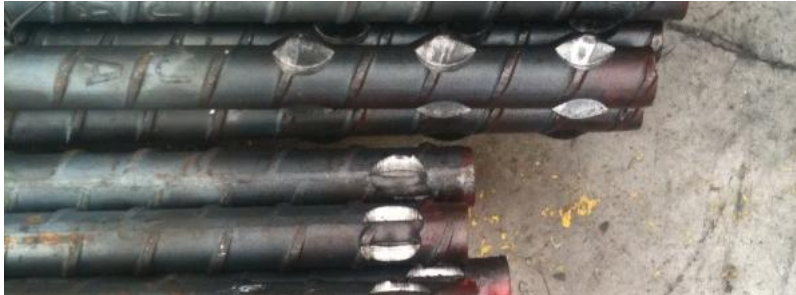
Figure 5 - Pinched ear bolt modifications
