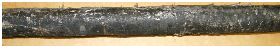
(c) 1 x 28 mm Pinched Ear, JLOK High Viscosity (thick) resin. Well shredded plastic film only 5 - 10 mm in size, well mixed entire along the entire length and colour indicating contact to the coal strata along the entire length.
