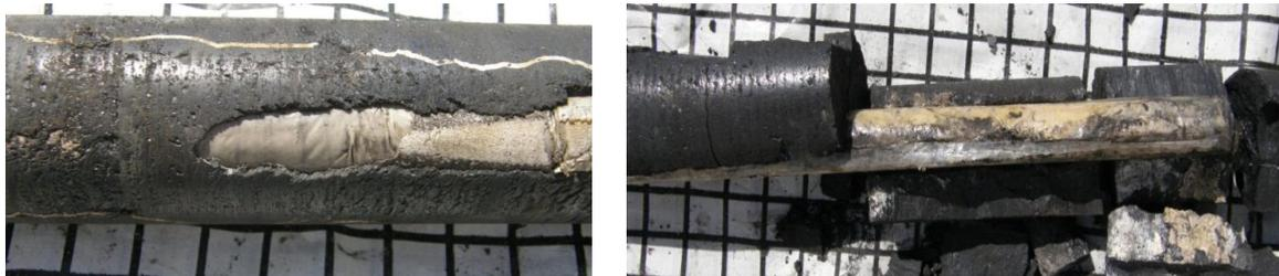
**Figure 1 - 1<sup>st</sup> site over-core: standard bolt, standard viscosity 2:1 water based catalyst resin**
