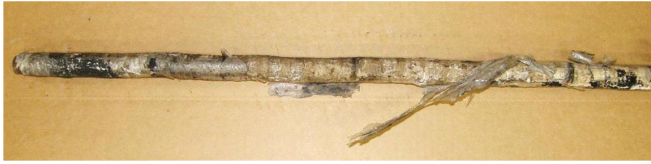
(a) 1 x 28 mm Pinched Ear, site 2:1 water based resin - extensive gloving with plastic film intact along 900 mm of bolt
