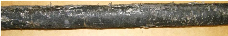
(c) 1 x 28 mm Pinched Ear, JLOK High Viscosity (thick) resin. Well shredded plastic film only 5 - 10 mm in size, well mixed entire along the entire length and colour indicating contact to the coal strata along the entire length.
