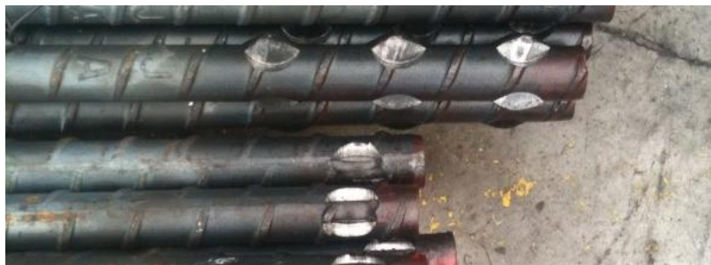
Figure 5 - Pinched ear bolt modifications
