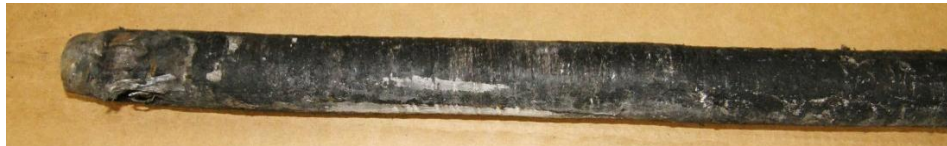
(b) Standard bolt, site 2:1 water based resin - extensive gloving with plastic film intact along 600 mm of bolt
