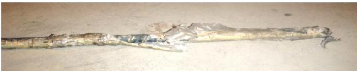
**Figure 2 - Overcored bolt taken from the support pattern**
