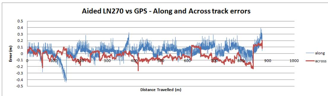
**Figure 6 - 2D position errors (orthogonal components of along track in blue and cross track in red) between the inertial navigation system and on-board RTK GPS equipment**
