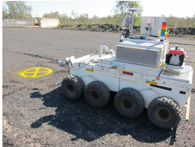
Figure 2 - Phoenix skid steer vehicle used to evaluate the performance of the inertial navigation systems
