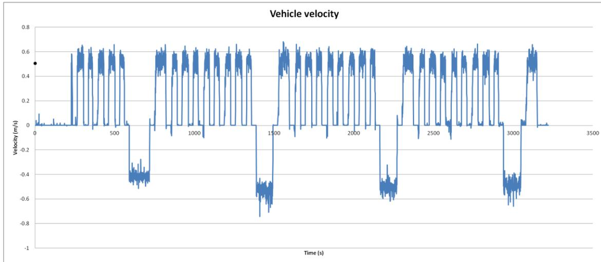
**Figure 5 - Phoenix velocity vs time plot to indicate the ZUPTs and forward/reverse motion during the two-heading mining plan**
