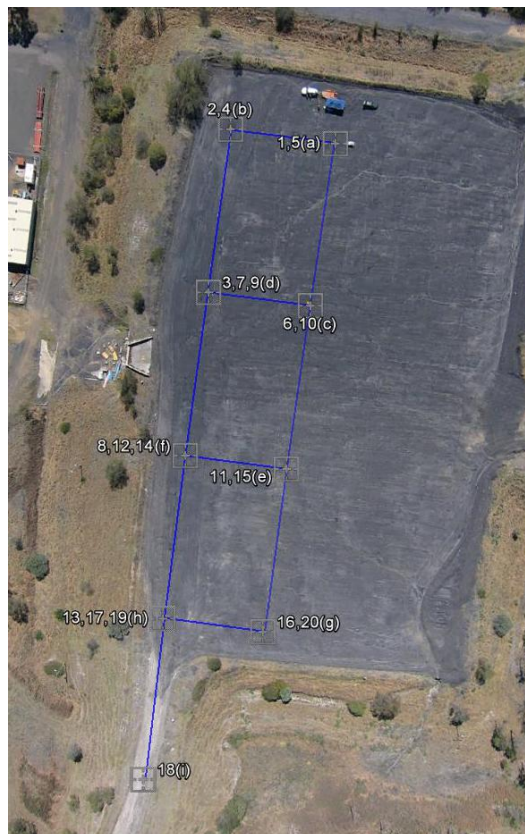
Figure 4 - Aerial view of Ebenezer test site with waypoints and mining plan shown
