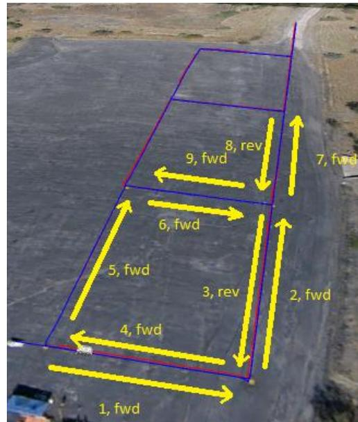
Figure 3 - Image showing two-heading roadway development mining plan
