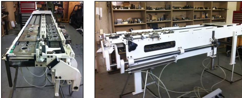
Figure 4 - Washer delivery system
