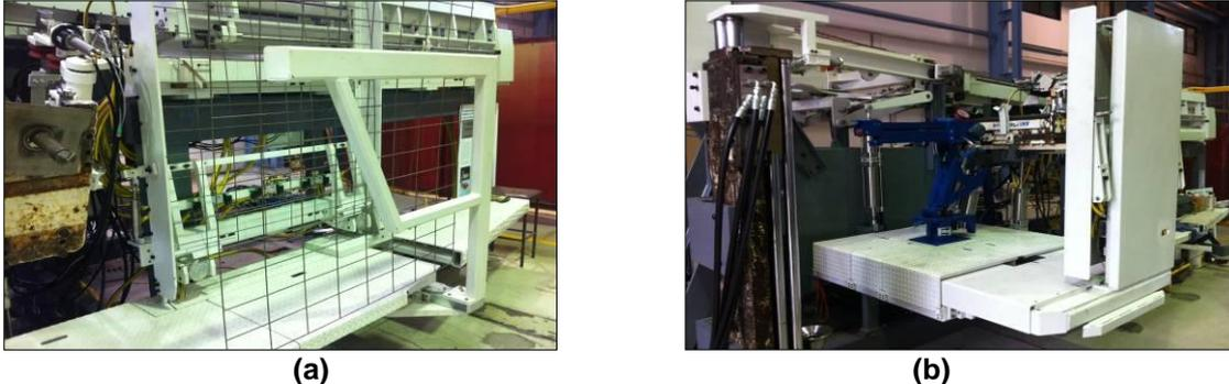
Figure 8 - Rib Mesh Manipulator: (a) cassette dispensing unit and transfer arm, and (b) crash barrier in the extended out position
