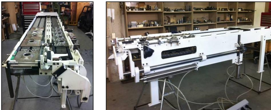
Figure 4 - Washer delivery system
